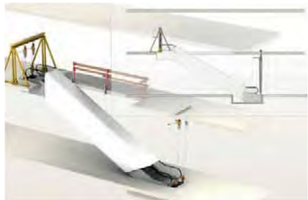
Figure 8.5 Installation using a lifting frame
