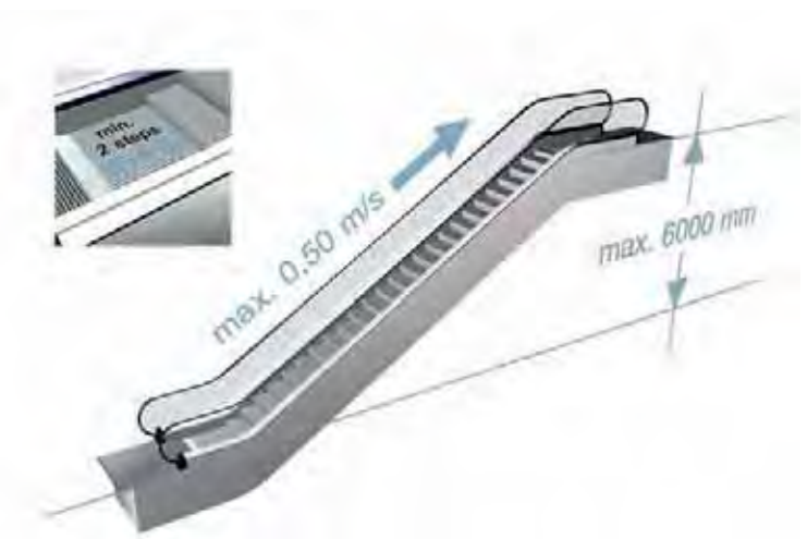
Figure 5.11 Vertical rise and speed of an escalator with two horizontal steps.
