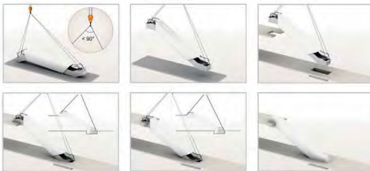
Figure 8.1 Installation in one complete section by a crane is probably the quickest and simplest method
